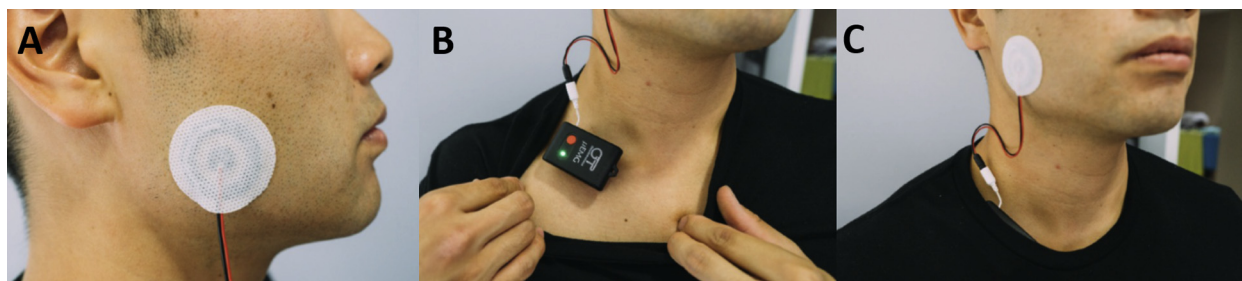
Fig 2. EMG portable data logger. A , Location of the concentric electrode on the right masseter; B , device positioned on the right clavicle; C , device and electrode in place.
